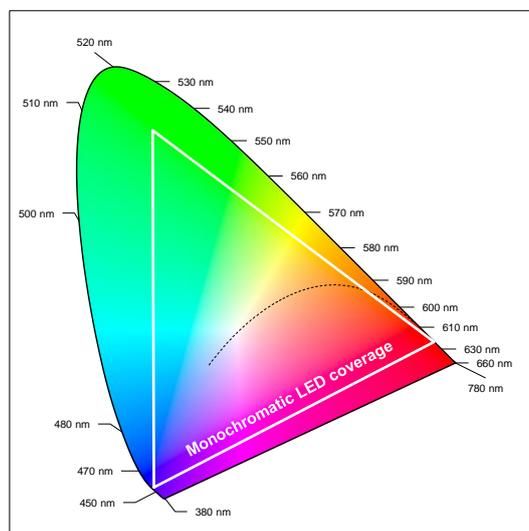
Figure 5. Monochromatic gamut in CIE 1931 diagram.
